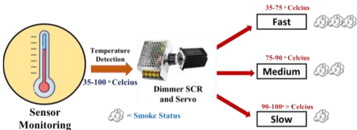
Fig. 10. Working scheme for silicon-controlled rectifier dimmer and revolutions per minute blower control system design.
