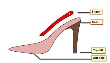
Fig. 18 Shank embedded in outsole-exploded view
