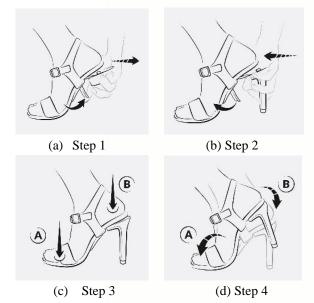
Fig. 3 Four steps of converting flat to high heel
