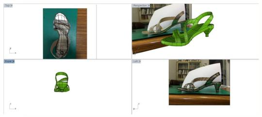
Fig. 17 Superimposed with flat shoe images and shoe model
