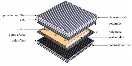
Fig. 1 Exploded View Diagram for LCD panel
